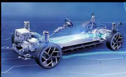
Safety - E-Platform 3.0 With The Cell-to-Body (CTB) Structure
